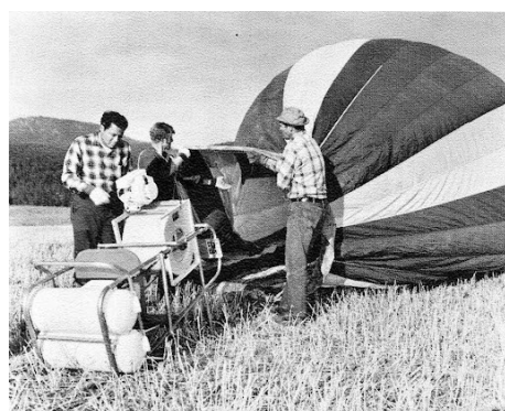
CHAIR ASSEMBLY THAT INCLUDED AN INFLATION FAN.
