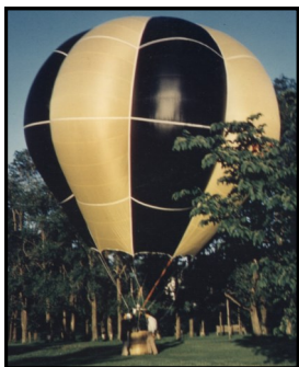
First eight gore and original bulbous balloon AX-3 balloon by Piccard in 1965
