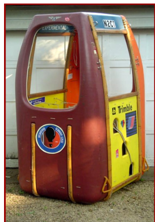
Early Don Piccard Balloons plastic BODY HELMET (basket) could carry up to 3 persons
